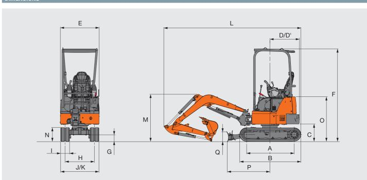
This illustration shows with 0.93 m arm, 0.044 m³ bucket and 230 mm rubber shoes and heavier counterweight 240 kg.
