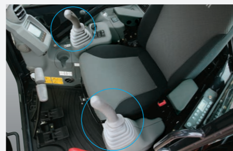
Control lever Shown equipped with cab, armrests, air conditioner, pedal and FM/AM radio as optional items.
